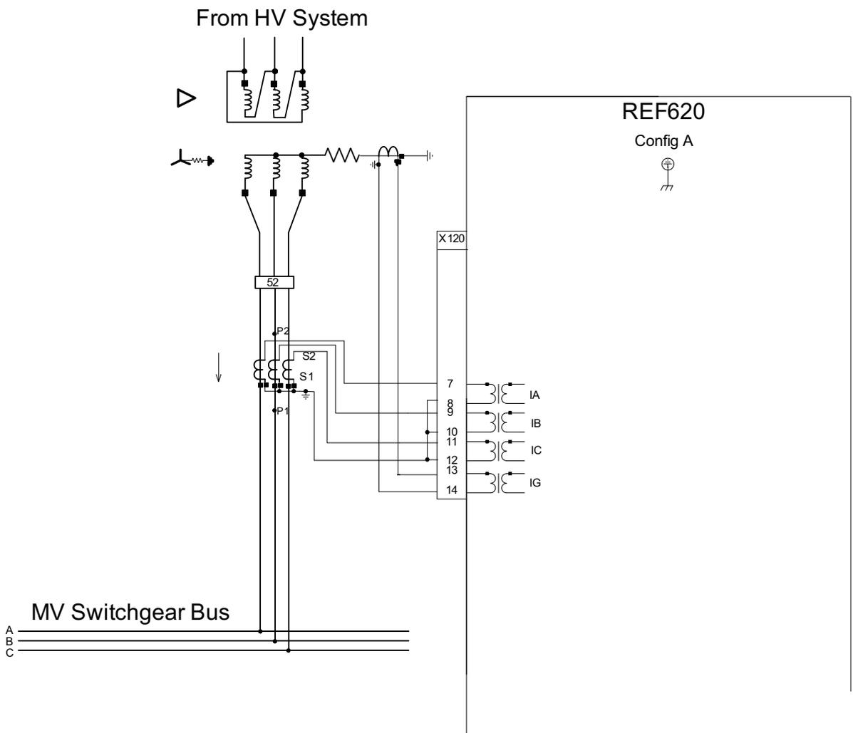
Figure 8. REF620 connection diagram config B
