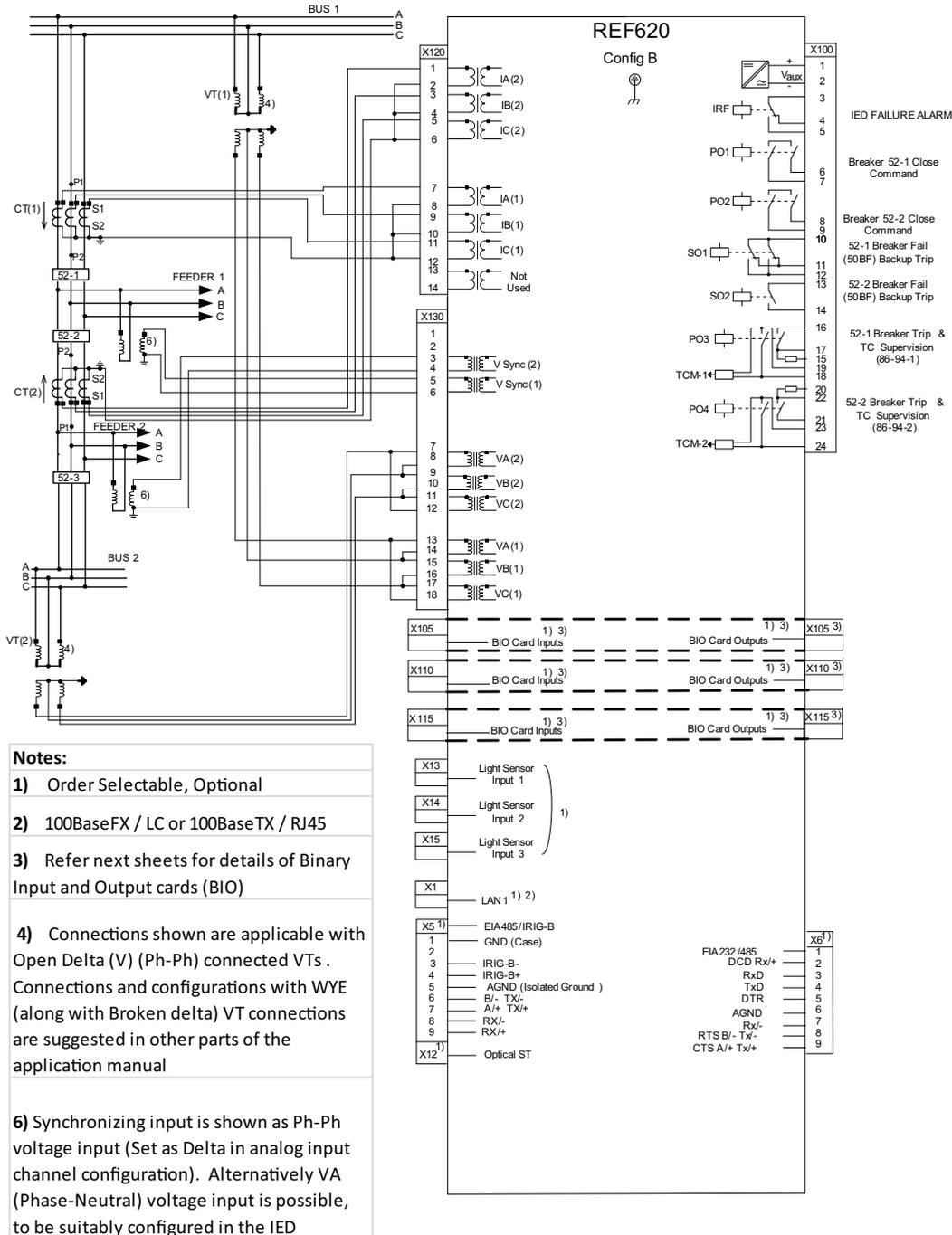
Figure 9. REF620 connection diagram config B
