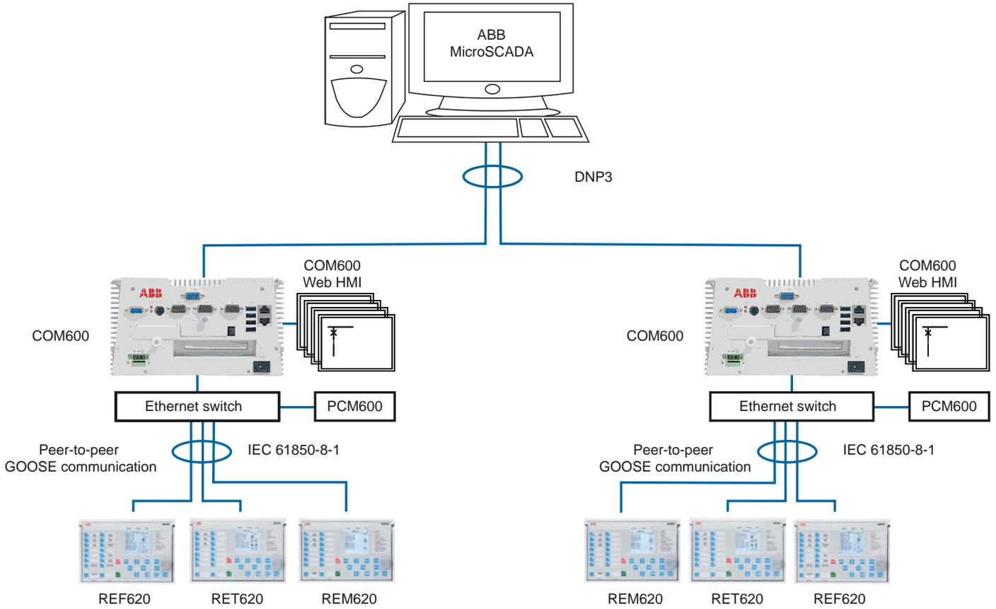
Figure 5. Industrial distribution network example using 620 series IEDs, Station Automation COM600 and System 800xA
