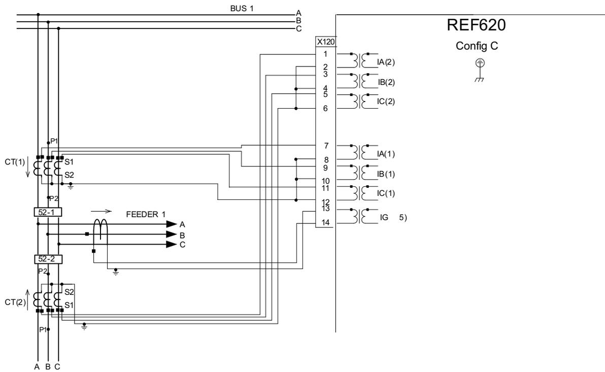
Figure 13. REF620 connection diagram config C
