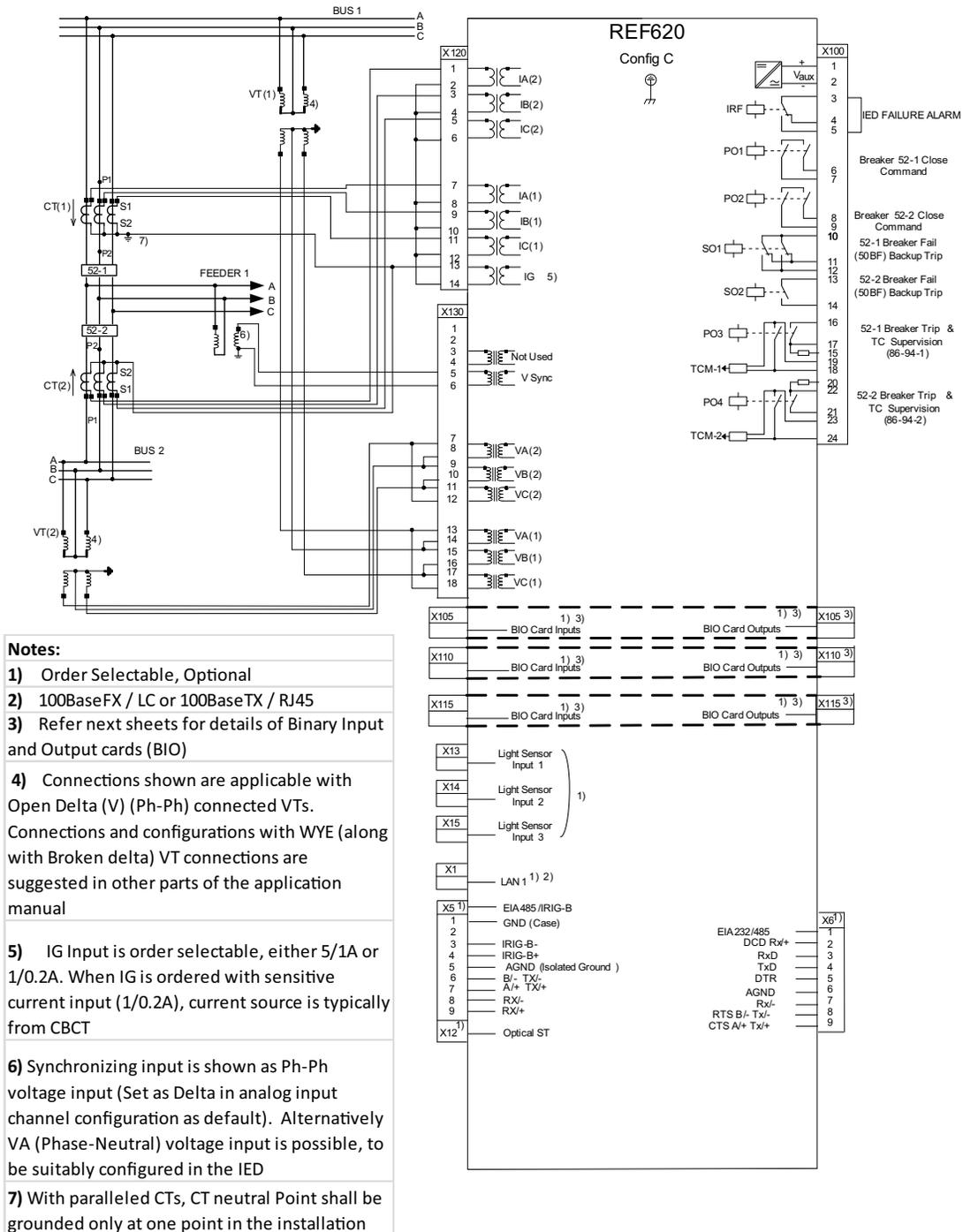
Figure 12. REF620 connection diagram config C
